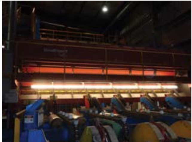
GradExpert: Opticaly grades for visual consistency and removes boards that fail to comply with this specification
